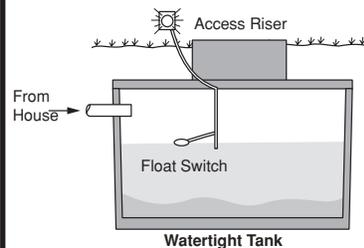
A holding tank is a large tank, similar to a single-compartment septic tank, that holds wastes discharged from a house, building, etc. The holding tank is designed to hold waste for a designated period of time. The tank requires pumping on a regular basis (weekly, bi-weekly, etc.), depending on the quantity of wastewater generated. An alarm will sound when the wastes in the tank reach a specified level that requires pumping the tank.
