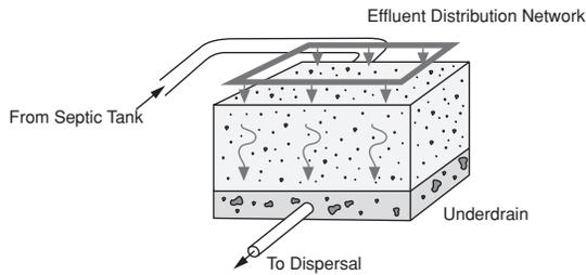
Filtration is a process whereby pollutants, primarily solids in suspension, are removed from water by physically trapping them in media containers called filters. Media can be sand, gravel, or alternative material that is permeable and allows water to pass through. Filtration consists of two common types: 1) single-pass filtration and 2) multi-pass filtration.
