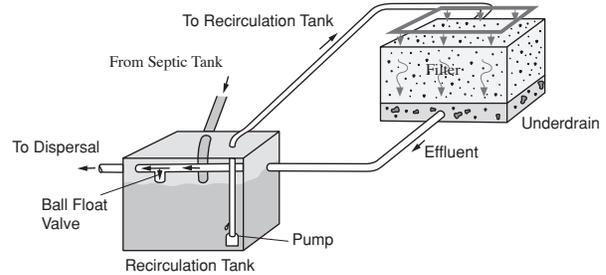
In multi-pass (recirculating) filtration, the water passes through the filter as it does in single-pass filtration except that when it reaches the filter underdrain, only a portion of the water is discharged for final dispersal. The remainder of the effluent is collected into a pump tank called a recirculation tank and goes through the filter again. The number of times the water passes through the filter is called the recirculation ratio and is determined by the desired quality of the effluent.
