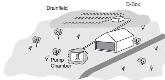
In a pressure assist drainfield, the wastewater is pumped to the field because it cannot flow by gravity. Wastewater flows from the septic tank to the pump chamber where it is pumped uphill and dispersed by gravity through the absorption field lines. Other than the addition of the pump chamber, this system operates identically to a septic tank-soil absorption system.
