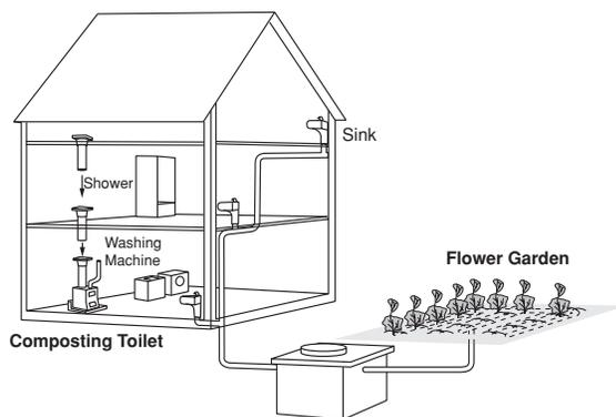
Wastewater coming from the house can be separated into two waste streams: blackwater and greywater. Wastewater from toilets is always considered blackwater and, depending on local guidelines, may also include wastewater from kitchen sinks. Greywater is the wastewater generated from other plumbing fixtures in the house, such as showers, bathtubs, dishwashers, washing machines and bathroom sinks.
