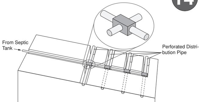
A serial distribution system utilizes a series of absorption trenches in succession. The pretreated effluent is usually gravity fed. However, some serial distribution systems may require a pump to move the effluent from trench to trench thus maximizing the infiltrative capacity of each trench before effluent flows from one trench to the next.
